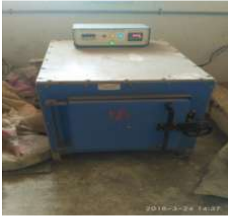
Fig.3.4: Heating of Concrete cube at 600 0 C
