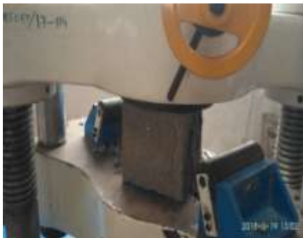
Fig.2.4 Testing of M20 grade of Concrete cube on UTM
