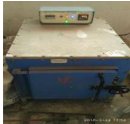
Fig.3.5: Heating of Concrete cube at 900 0 C
