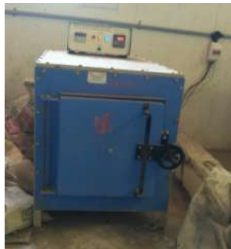
Fig.3.3: Heating of Concrete cube at 300 0 C
