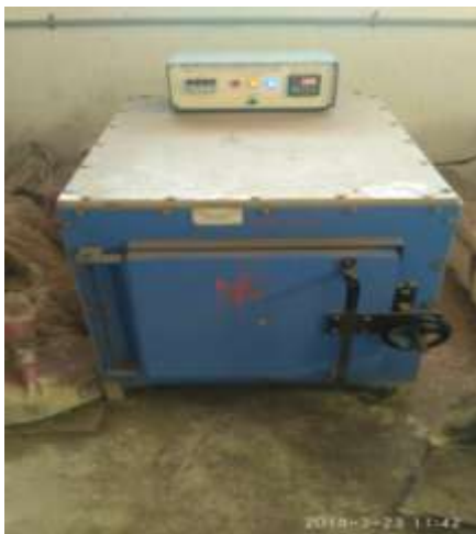
Fig.3.2: Heating of Concrete cube at 100 0 C
