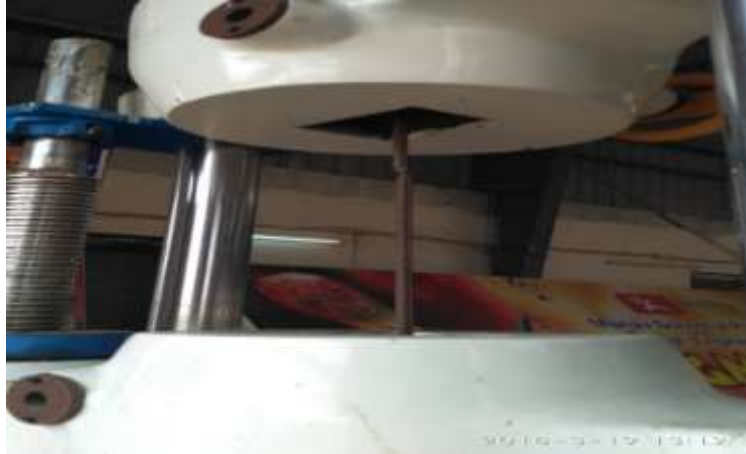
Fig.2.6 Tensile testing of Reinforcement Steel
