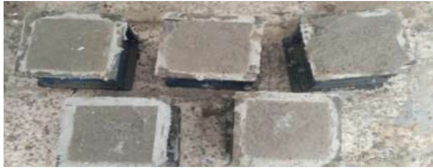
Fig.2.3: Concrete cubes of M30 grade
