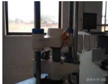
Fig.2.5 Testing of M30 grade of Concrete cube on UTM
