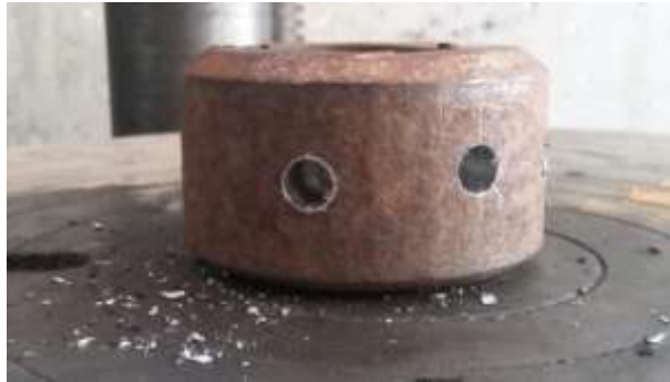
Fig. 7: Image shows drilled hole on workpiece for setup of 30° angle.
