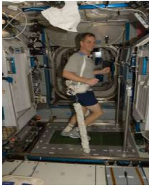
Fig. 2: NASA astronaut T.J. Creamer, Expedition 22 flight engineer, equipped with a bungee harness, workouts on the Combined Operational Load Bearing External Resistance Treadmill (COLBERT) in the Harmony node of the International Space Station.
