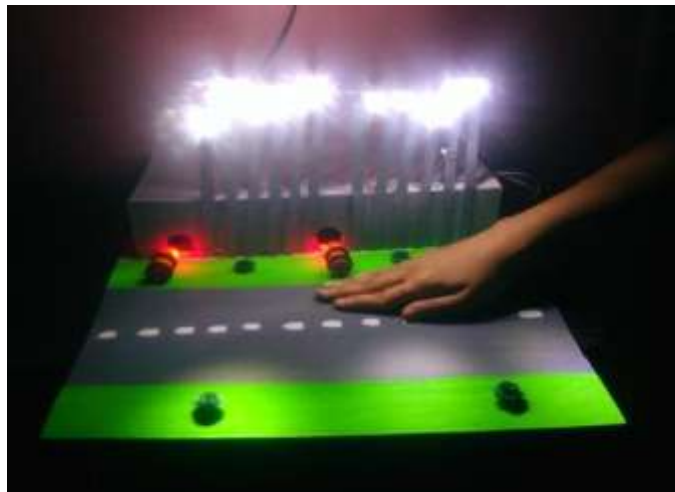
Fig. 2 Street Light glows with 100% intensity when obstacle is detected
