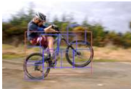
Fig: 6 Bicycle Detection in an image
